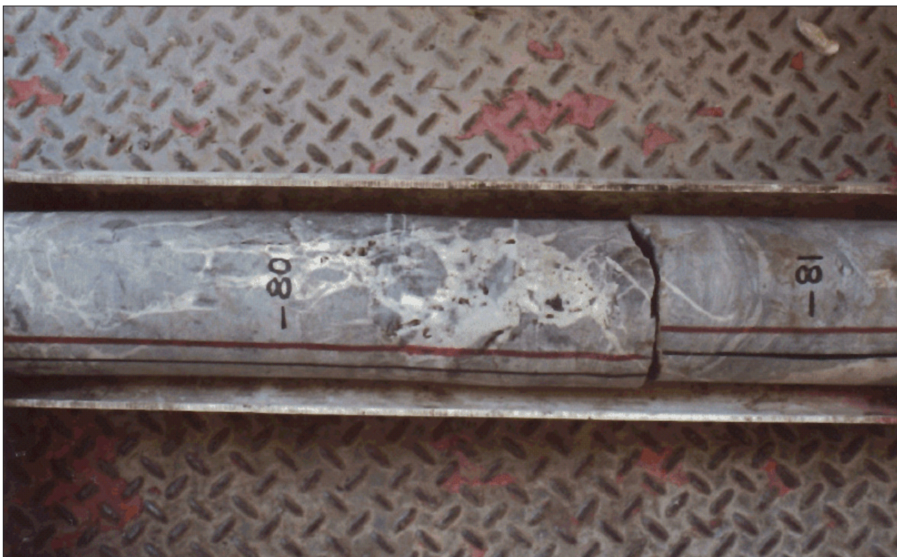
Figure 3b. Core #3 (uncut) from 14,280-81'. Note large open porosity in quartz- and calcite-filled fracture zone.
