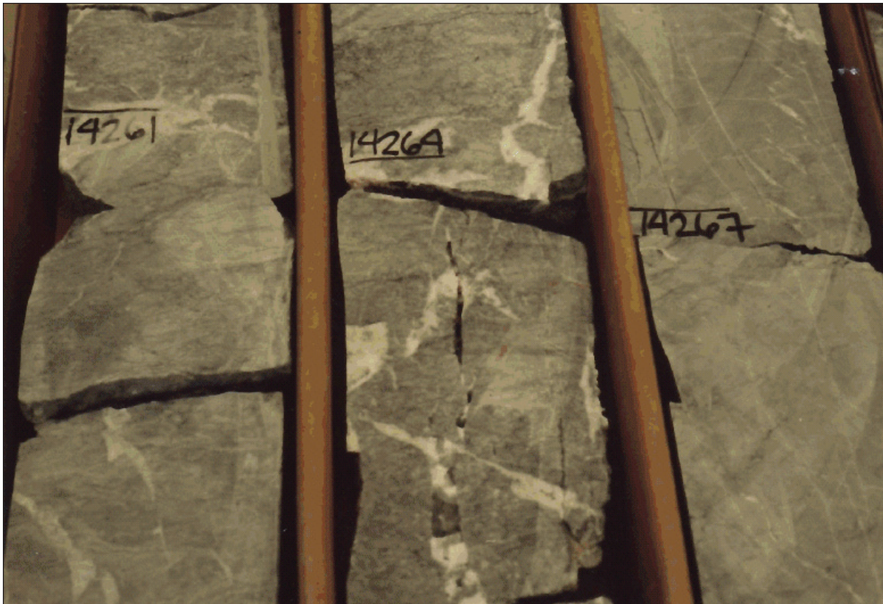
Figure 3a. Core #3 (slab). Note that at 14,264' there numerous large, open fractures with partial quartz and calcite filling while at 14,261' and 14,267' only minor fracturing is observed. The samples at 14,264' are coarse- to medium-crystalline metadolomite while at the other depths the samples are very fine crystalline metadolomite.
