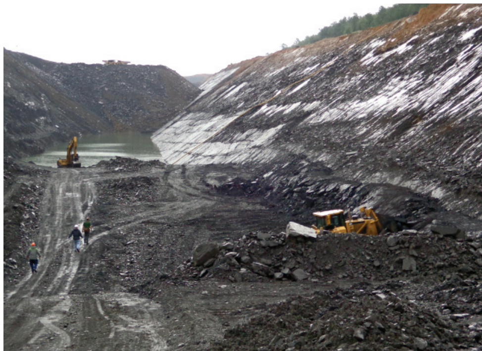
Figure 2. View looking east of coal geologists in Farrell-Cooper Mining Company Bull Hill surface coal mine in Le Flore County, Oklahoma. Steeply dipping (37° north dip) Lower Hartshorne coal is at the base of the high wall in the right side of the photograph.
