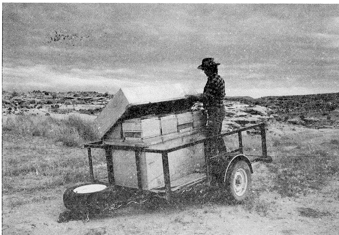
Figure 10. Custom-made portable washing tanks. These tanks have a collective soaking capacity of 24 boxes; when fitted together for shipment, 32 boxes can be accommodated.
