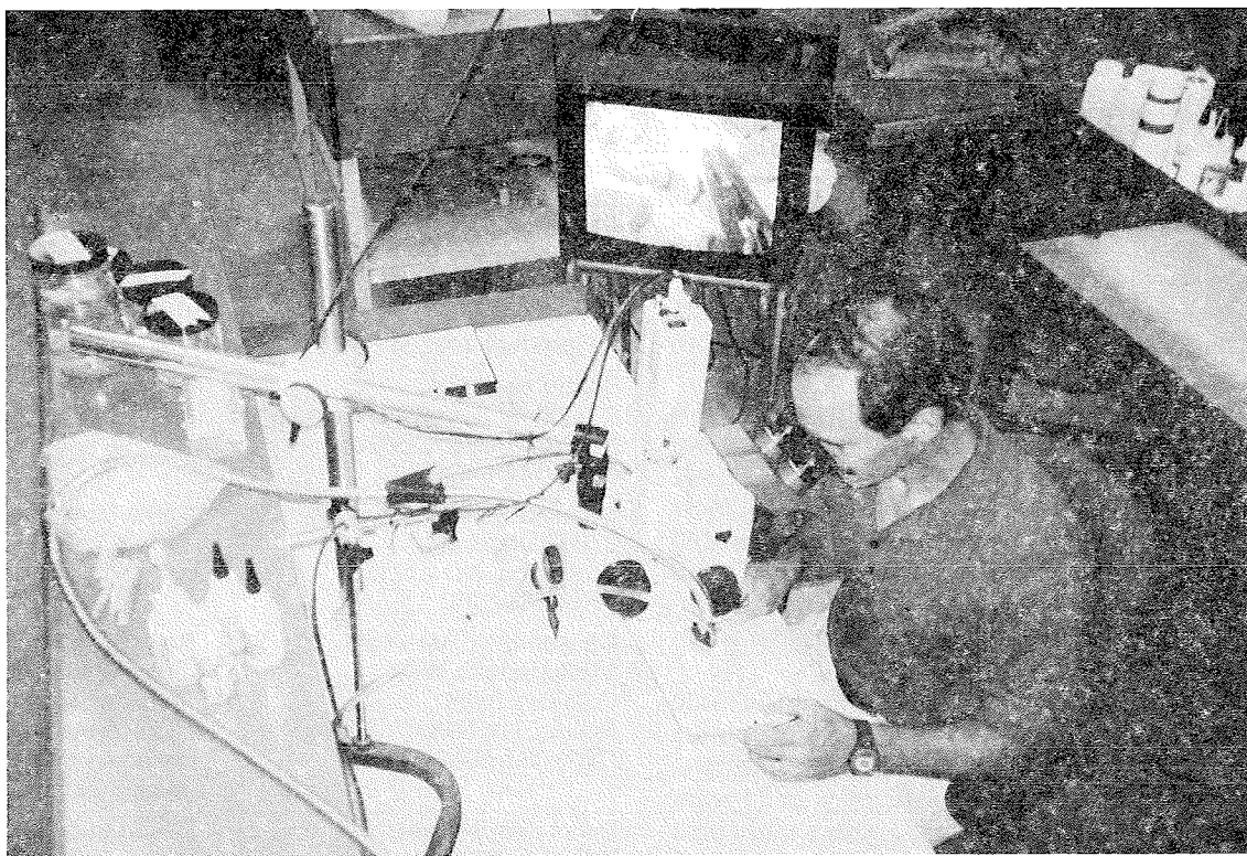
Figure 1. Binocular microscope configured for micropreparation. The scope is mounted on a long boom, permitting a wide range of movement of specimens, materials, and equipment; the boom is supported on a heavy stand for stability. The light source is a twin-pipe fiber-optic system with a long basal pipe, so that the light source itself is placed well out of the way; a clear plastic air tube, for blowing dust and small particles, is affixed to the left pipe. This microscope is configured with a trinocular head, to which a video camera is mounted. The image can be viewed via a monitor (background, center). The camera and monitor are useful for teaching preparation techniques, as well as for consultation for the study or conservation of specimens, exhibition, and for other purposes.
