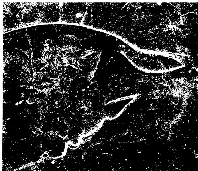
Figure 18. Negative print of acetate peel showing poorly washed grainstone of St. Clair Limestone, Batesville Stone quarry. Note unfragmented trilobites and sparry calcite (dark grains) in protected areas. Bar is 2 mm.
