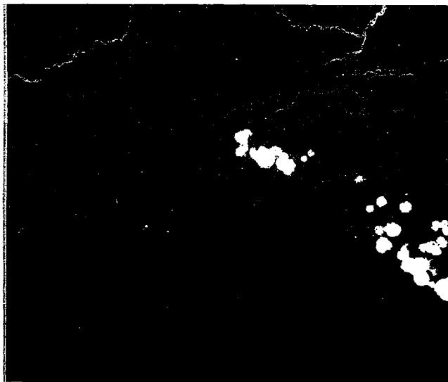
Figure 17. Negative print of thin section showing basal ostracode wackestone of St. Clair. White areas are pyrite. Bar is 1 mm.
