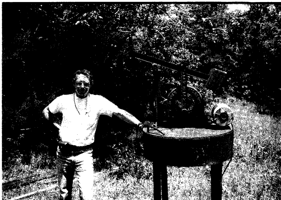
Author stands by small, electrically powered pump jack in the central part of Redden oil field. Well is probably the Croxton no. 2 Miller, from which ~50 bbl of 41 gravity oil was produced in early 1986. Reservoir is in Stanley Group, ~72 ft below the surface. Oil storage tank in right distance. Ticks everywhere. (Photo by Neil Suneson, June 1989.)
