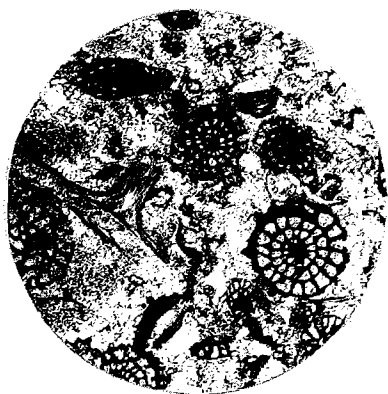
Figure 48. Fusulinid calcilutite from limestone bed II of Buckhorn area (Stop 8). Micrite matrix is partly recrystallized into microgranular calcite. \times 12.5 .
