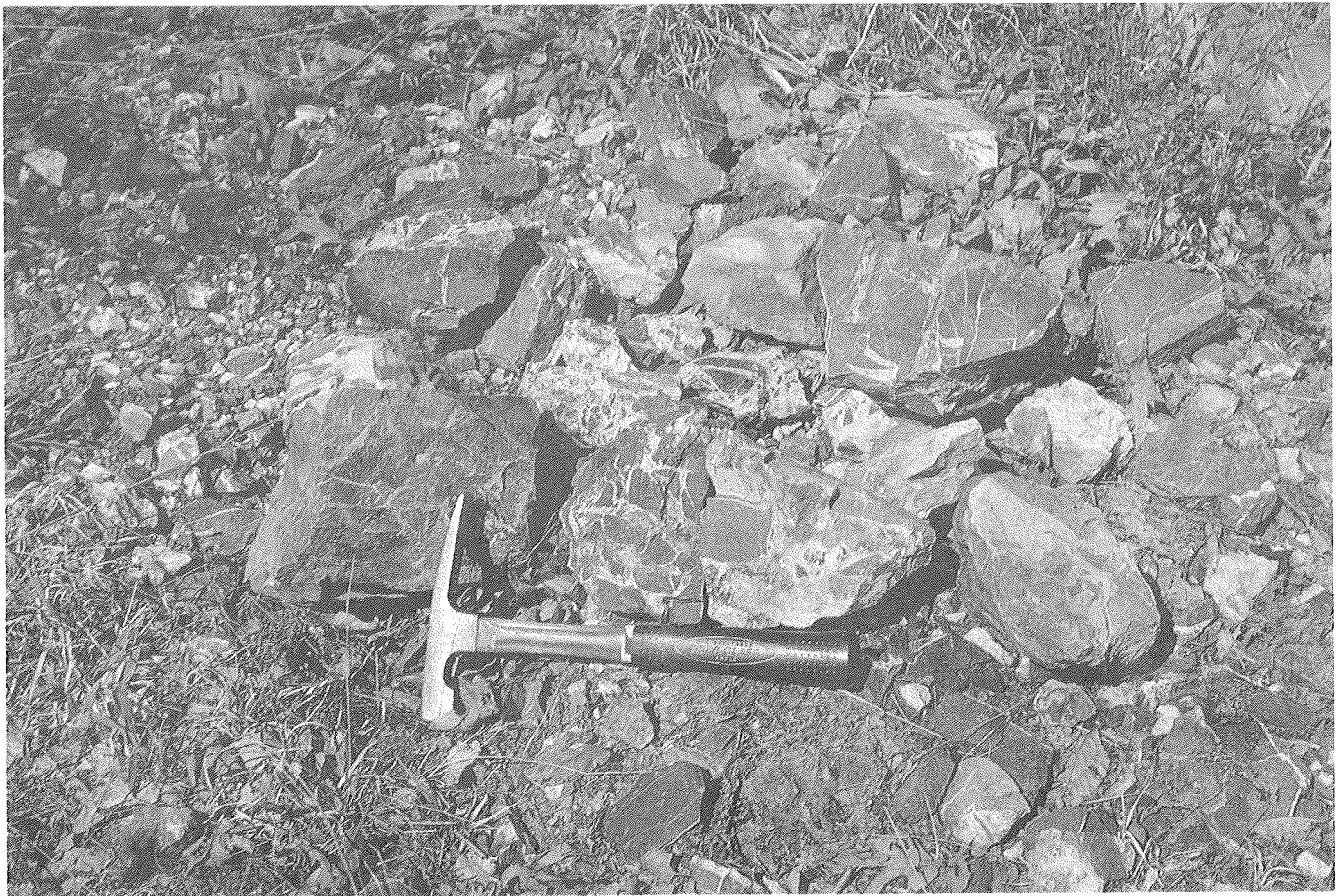
Figure 21. Going prospect. Closeup view of brecciated quartzite and phyllite, with quartz, sphalerite, and galena, from tailings in SE 1/4 SE 1/4 NW 1/4 sec. 28, T. 1 S., R. 26 E., McCurtain County, Oklahoma. Main tailings are northwest of north pit. April 11, 1973.
