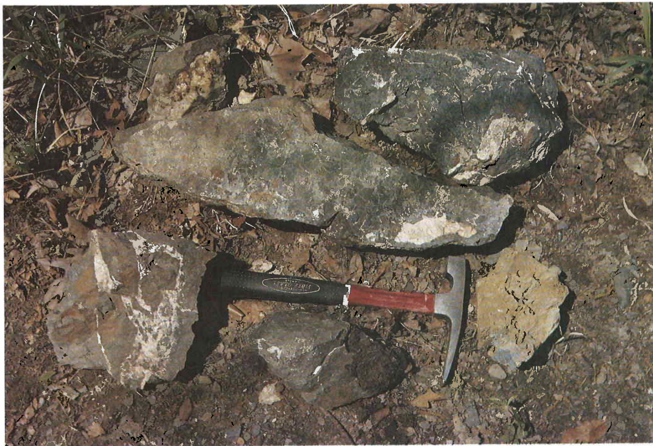
Figure 14. Buffalo Mine. Sphalerite and galena in brecciated quartz veins in Stanley phyllite and quartzite, on Mine Creek about 100 ft north of Buffalo Creek, in NE \frac{1}{4} NE \frac{1}{4} SW \frac{1}{4} NW \frac{1}{4} sec. 14, T. 2 S., R. 26 E., McCurtain County, Oklahoma. April 11, 1973.
