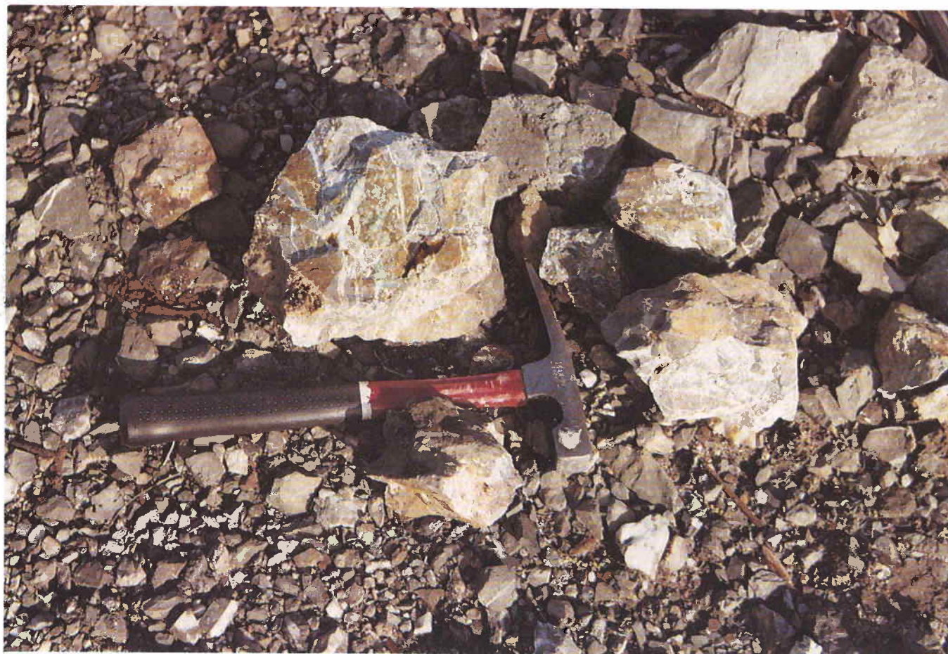
Figure 33. Davis Mine. Samples of sphalerite in quartz veins in Stanley quartzite and phyllite, from tailings, near CSE \frac{1}{4} NW \frac{1}{4} NW \frac{1}{4} sec. 10, T. 7 S., R. 32 W., Sevier County, Arkansas. April 11, 1973.
