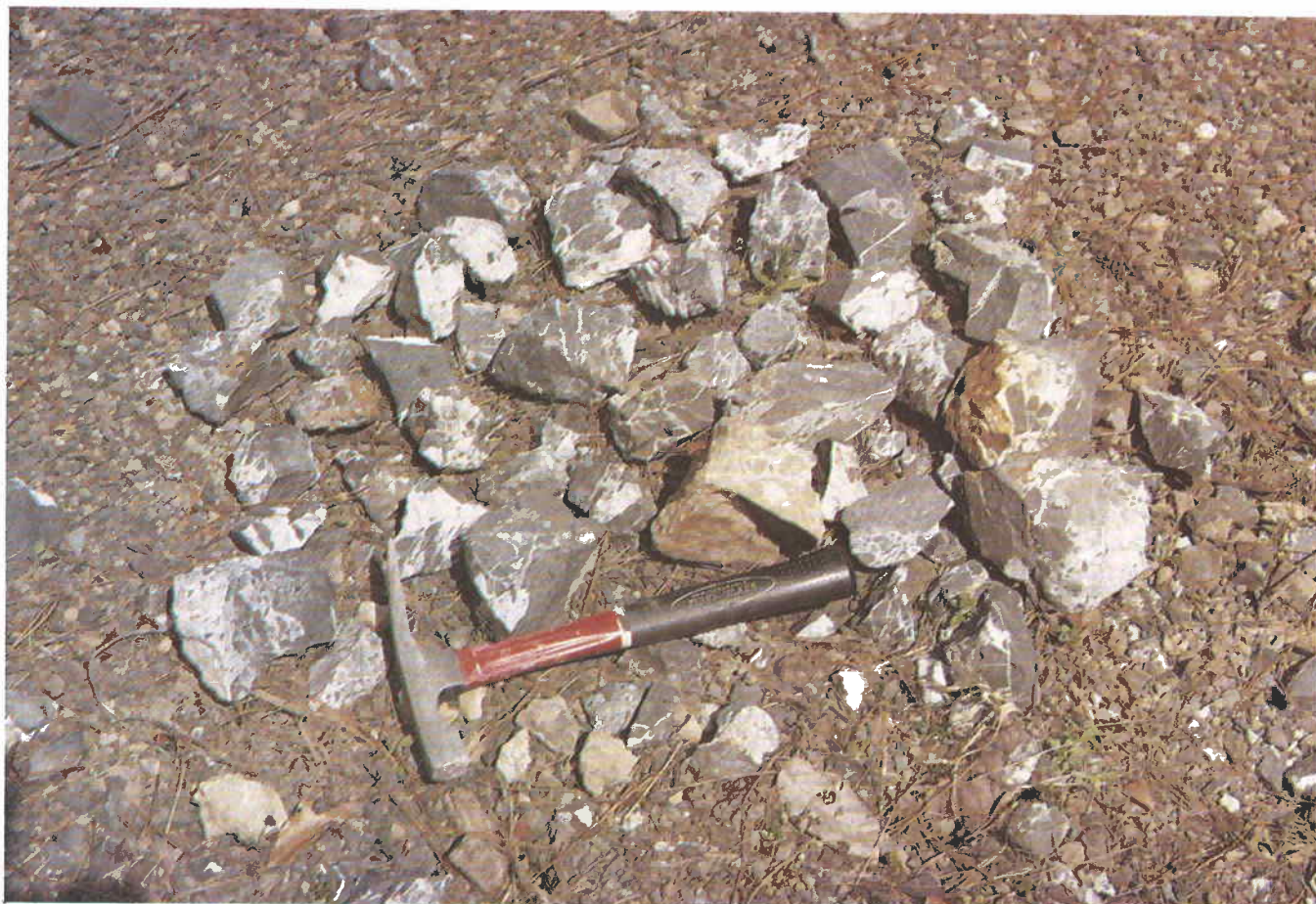
Figure 17. Duncan prospect. Closeup view of sphalerite and galena in quartz veins in Stanley phyllite and quartzite. Vein strikes N. 60° E. and dips 40° NW., in SE \frac{1}{4} NE \frac{1}{4} NW \frac{1}{4} SW \frac{1}{4} sec. 10, T. 2 S., R. 26 E., McCurtain County, Oklahoma. April 11, 1973.
