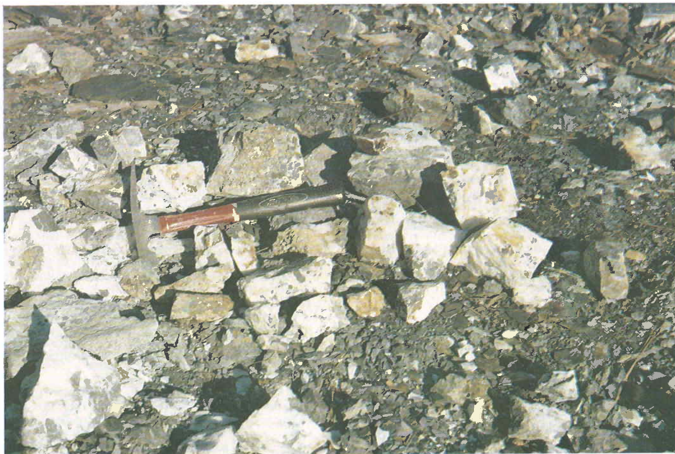
Figure 26. Bellah Mine samples: sphalerite, galena, chalcopyrite, and malachite in quartz veins, from tailings, in SE \frac{1}{4} NW \frac{1}{4} sec. 27, T. 7 S., R. 32 W., Sevier County, Arkansas. April 10, 1973.
