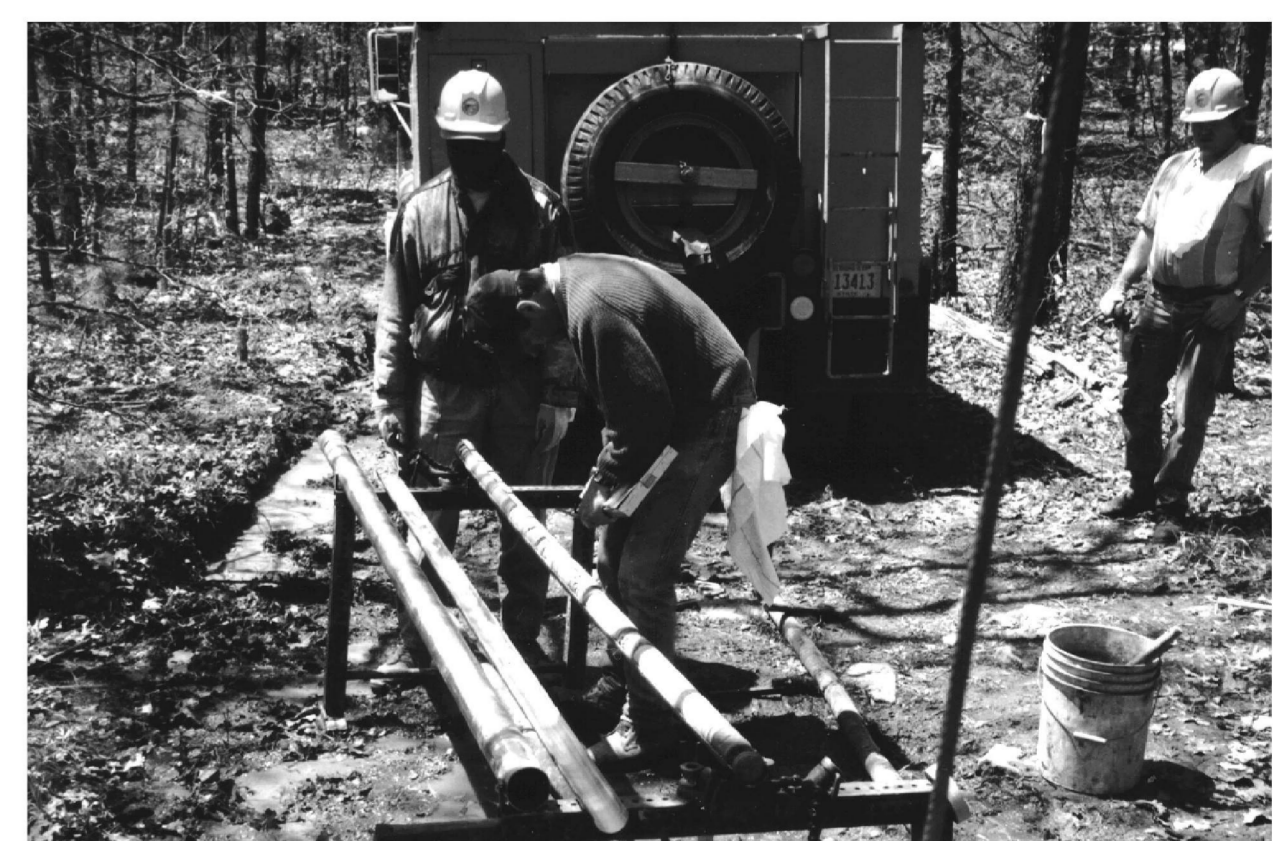
Oklahoma Department of Transportation crew logging core at the site of C-SH 82-boring 3.
