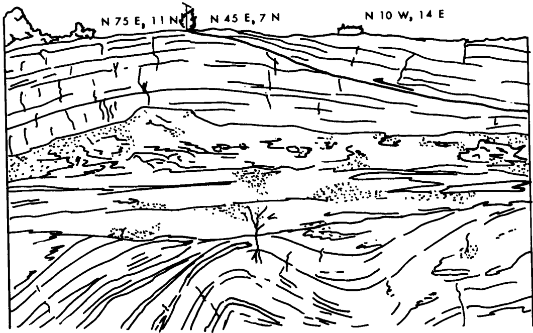
Figure 40. Diagrammatic sketch of quarry showing the low-angle thrust fault in the upper level of the quarry and typical Arbuckle-type folding style of beds in the lower level of the quarry (see Figs. 41,42). Stop 5.
