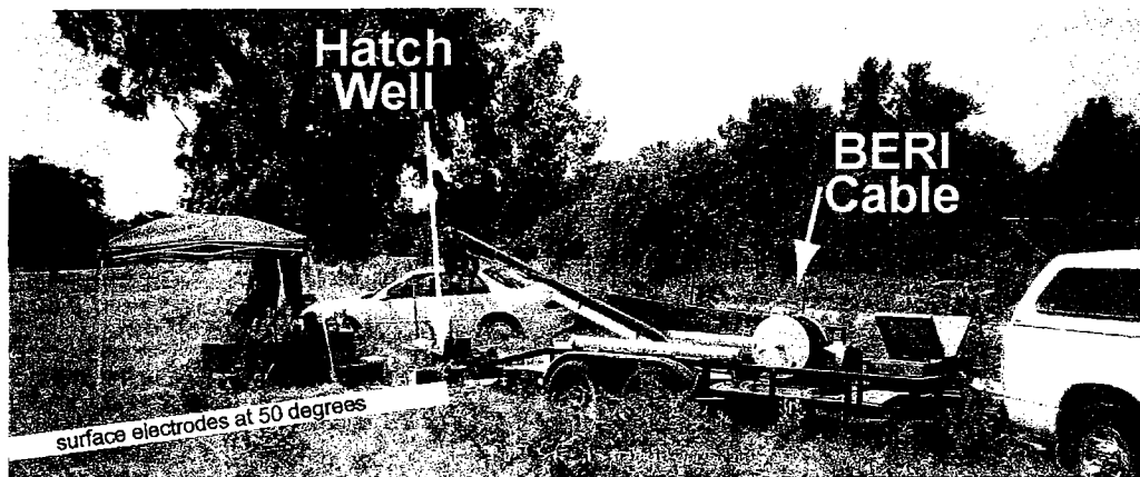
Equipment setup at Hatch well site for ERI image at orientation of 50 degrees. Picture is taken from the north looking south.
