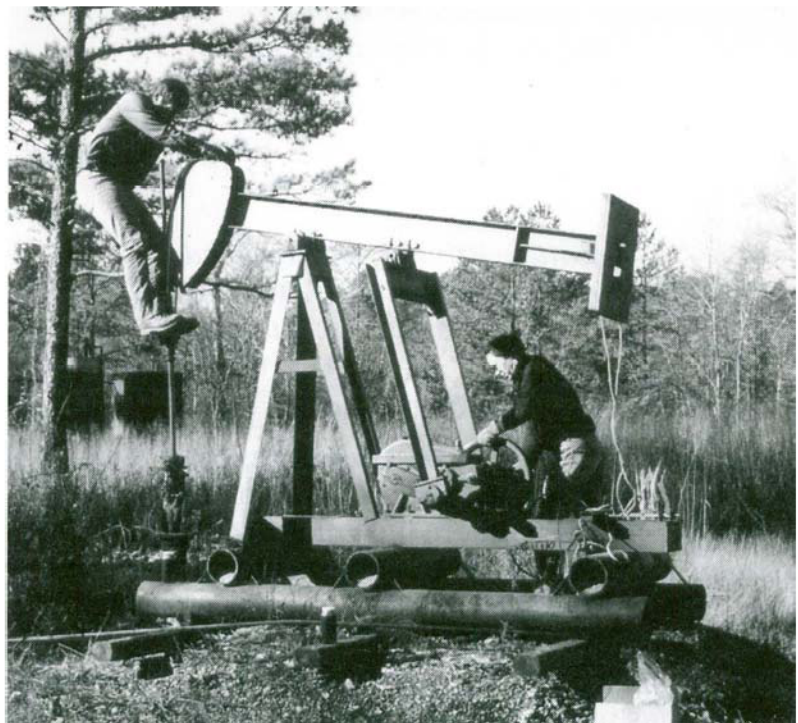
Figure 17: Neil Suneson and Jock Campbell (Oklahoma Geological Survey) hand-operating the pumpjack on the Select No. 1 Warren, December 5, 1988. After 45 minutes of back-breaking labor, oil was recovered. This method of oil collection is not recommended. (from Suneson, 2005)
