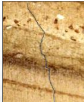
Mineback photograph (and line drawing) of fracture kinking, offsetting, and turning as interface is crossed (Warpinski, 2012)
