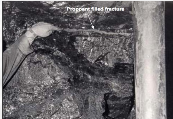
Proppant filled re-oriented horizontal fracture near the interface (Daneshy, 2009)
