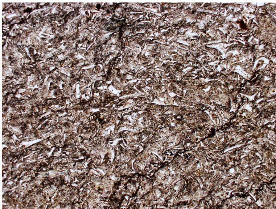
Figure 12. Photomicrograph showing silicified bubble-wall shards in tuff interbedded between rhyolite flows exposed northwest of Bally Mountain. Plane-polarized light; field of view ~5 mm across.
