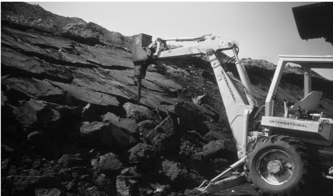
Photograph by Samuel A. Friedman showing a hydraulic impact pick, producing boulder size chunks of the Hartshorne coalbed at the Karsh Pit, McCurtain Number 2 surface mine, Great National Corp. (see p. 41-43).
