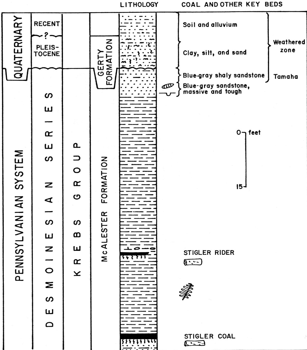
Figure 13. Generalized geologic column showing the exposed lower part of the McAlester Formation overlain by unconsolidated sand and clay in the areas of Porum, Muskogee County, and Stigler, Haskell County. Stigmaria are present in underclaystones, and abundant leaf compressions are present in shale in the interval between the two coals. (See Fig. 15).
