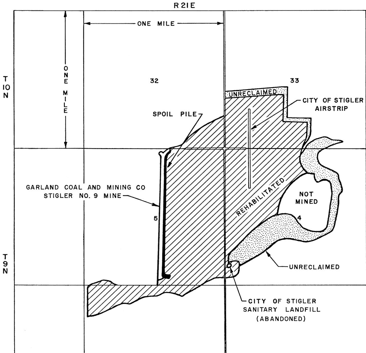
Figure 16. Map showing location of active pit and reclaimed areas at the Stigler No. 9 mine of Garland Coal and Mining Co.
