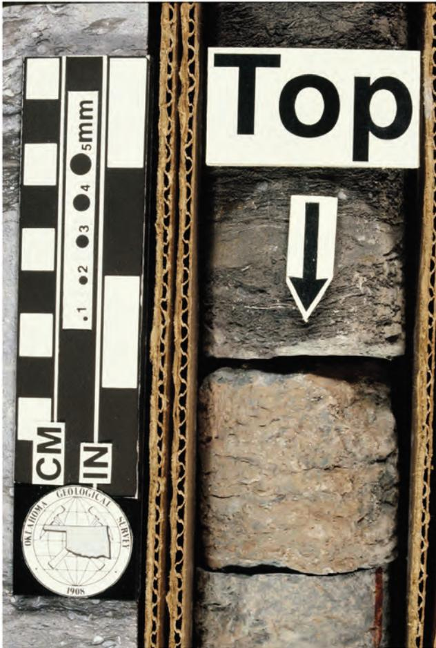
**Figure 9.** Sharp contact between transgressive marine facies of the Wreford Limestone above and regressive marginal-marine facies of the Speiser Shale below. Core hole KC-5, depth, 346.6 ft, Kay County, Oklahoma.
