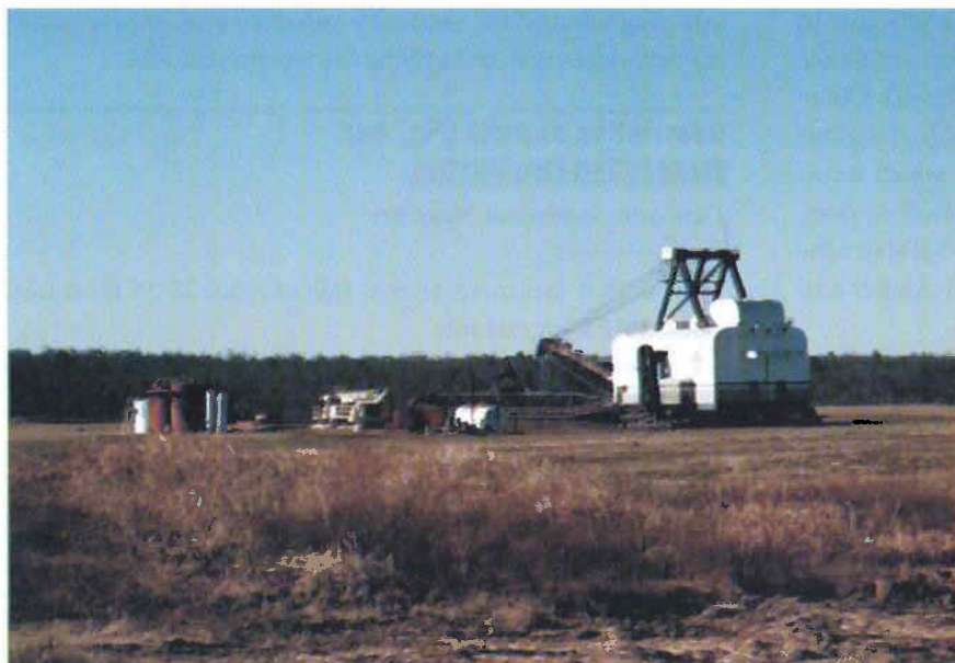
Figure 43. Drag line used by Farrell-Cooper Coal Company (from Suneson and others, 2005, fig. 104). Farrell-Cooper strip-mined the McAlester coal in its Red Oak South mine. The area is now completely reclaimed.
