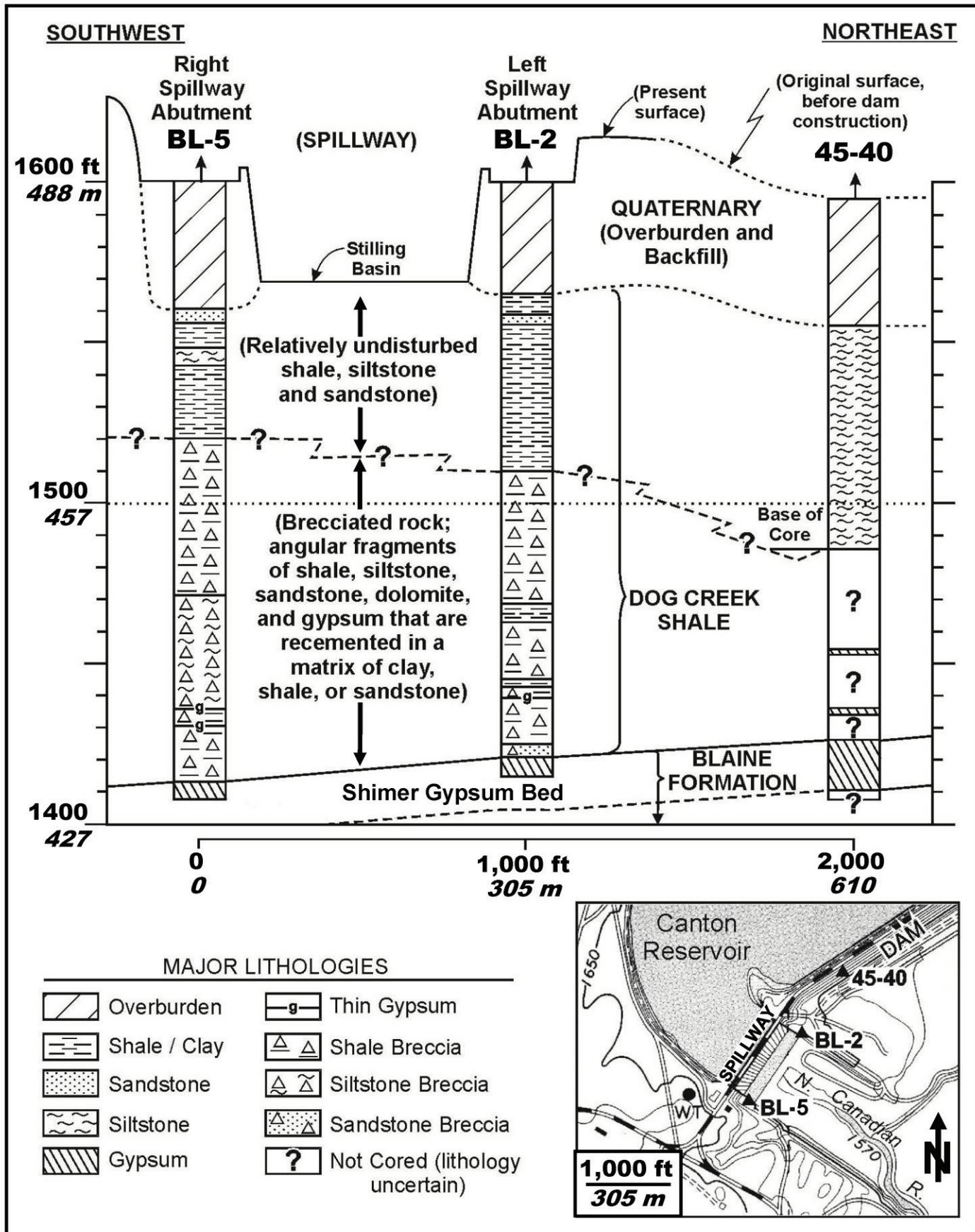
Figure 6. Cross section showing major lithologies beneath Canton Dam and spillway. View looking upstream, to the northwest. Boreholes BL-2 and BL-5 drilled in 2002-2003; borehole 45-40 is borehole #45 drilled in 1940 (before the dam was constructed). Location map shows present dam, primary spillway, and reservoir.
