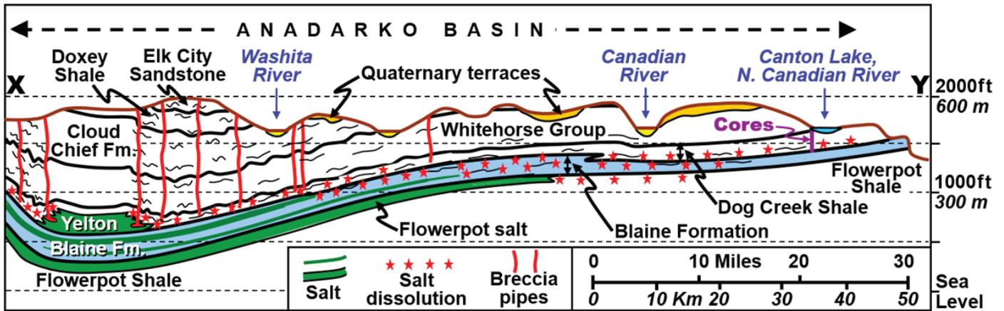
Figure 3. Cross section X--Y from axis of Anadarko Basin (left) to the northern shelf area (right). Permian salt units, still present in the deep subsurface, are dissolved at shallower depths, causing brecciation and collapse of overlying strata. Breccia pipes, shown schematically, locally reach the present land surface and contain blocks of Permian and Cretaceous strata. Location of cross section shown in Figure 1.
