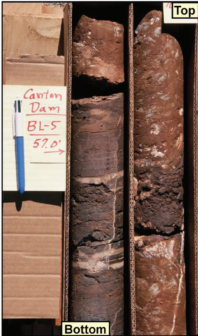
**Figure 7.** Core of Dog Creek Shale in borehole BL-5 on right spillway abutment. Core shows both fairly well-bedded and relatively undisturbed brown-gray shale (on left), and mottled red-brown and light-gray shale and siltstone with some small fragments of other rock types (on right). Length of pen is about 6 inches (about 15 cm).
