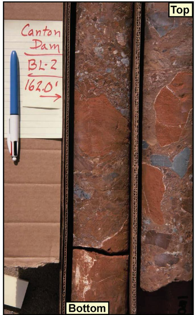
**LEFT: Figure 9.** Core of brecciated Dog Creek Shale in borehole BL-2 on left spillway abutment. Angular fragments of red-brown and gray shale, siltstone, dolomite, and gypsum are recemented in a matrix of red-brown shale and clay. **RIGHT: Figure 10.** Core of brecciated Dog Creek Shale in borehole BL-2 on left spillway abutment. Angular fragments of red-brown and gray siltstone and shale are recemented in a matrix of red-brown shale and clay.
