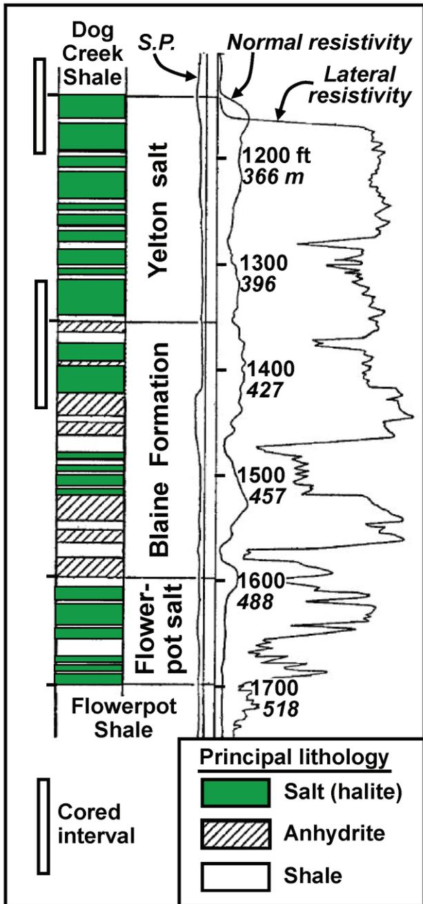
Figure 2. Salt beds are fully developed in the Blaine Formation and associated strata in the deep part of the Anadarko Basin. Lithology based on cores and log interpretation of Shell Oil Co. wells #1 Yelton and LPG-#1 Yelton, sec. 15, T.10N., R.21W., Beckham County, Oklahoma. After Jordan and Vosburg (1963).
