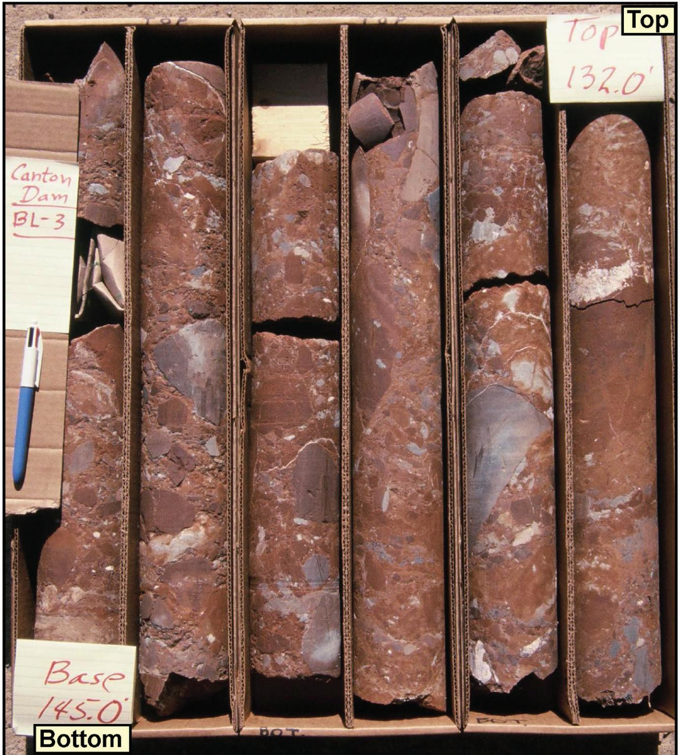
Figure 11. Three boxes containing 13 feet of core from borehole BL-3, drilled 40 feet from BL-2 on left spillway abutment. Top is 132.0 feet, and bottom is 145.0 feet. Core shows brecciated Dog Creek Shale, with fragments of shale, siltstone, dolomite, and gypsum that are recemented in a matrix of clay, shale, and sandstone.
