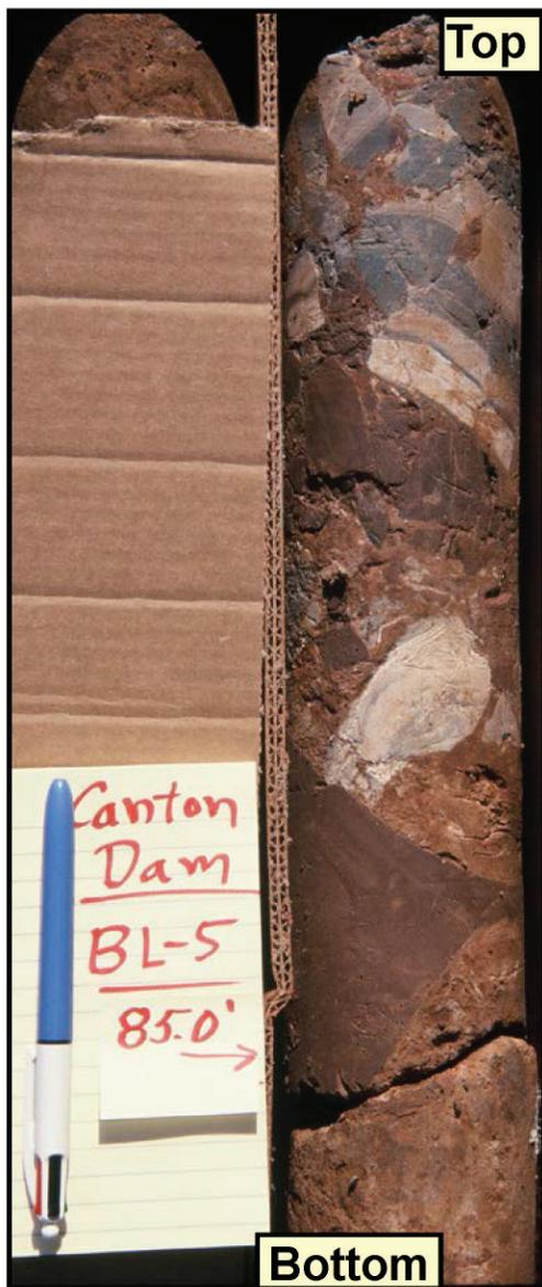
**Figure 8.** Core of brecciated Dog Creek Shale in borehole BL-5 on right spillway abutment. Angular fragments of red-brown and gray shale and dolomite are recemented in a matrix of red-brown shale, clay, and sandstone.
