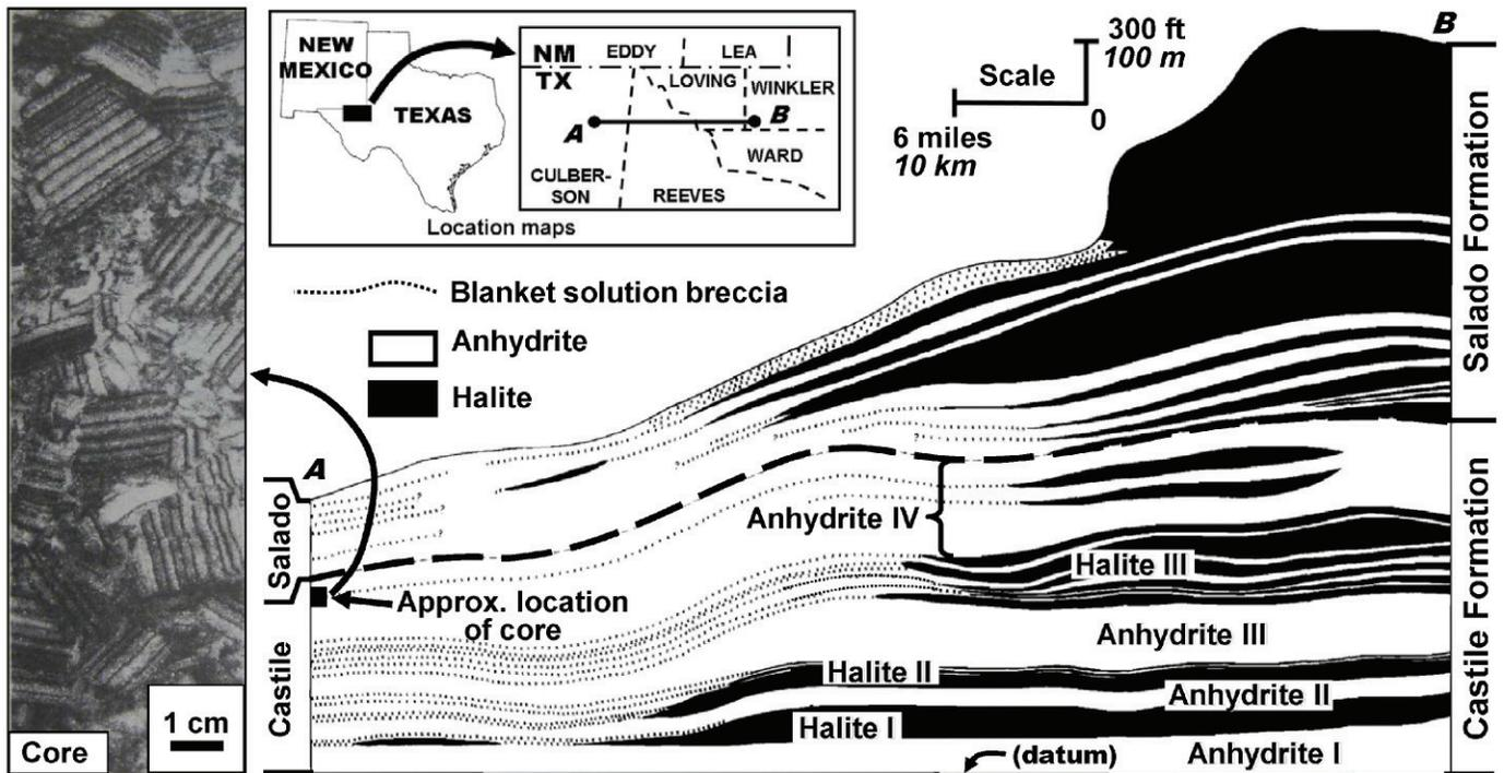
Figure 14. Schematic stratigraphic cross section A-B of Castile and Salado Formations in Delaware Basin of west Texas showing "blanket solution breccia" units where salt beds are dissolved towards the west, in the shallower, up-dip portion of the basin. On the left is part of a core showing collapse breccia caused by dissolution of salt and resultant collapse of overlying strata in the upper part of Anhydrite IV. Modified from Anderson and others (1972).
