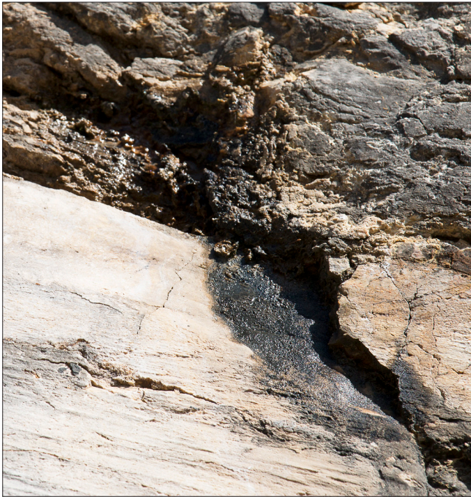
Figure 13. Water is seen flowing out of cracks in the outcrop at the location of the rockfall in October 2016.
