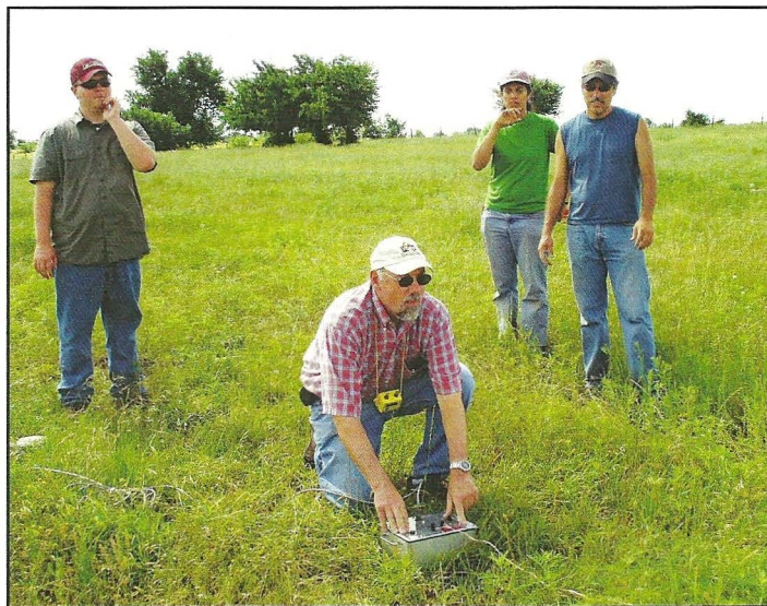
Randy triggering an active seismic source, 2007.
