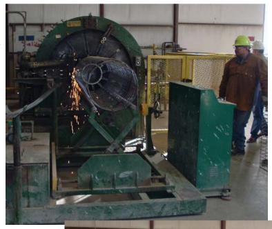
inforced steel cage for concrete pipe manufacture. (Photograph by Stan Krukowski, OGS.)
