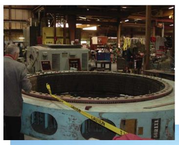
Figure 3. OKAA field trip at Evans Enterprises. Giant motor being repaired is from an OKAA member manufacturing plant's ball mill. (Photograph by Stan Krukowski, OGS.)
