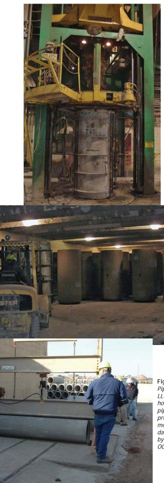
Figure 1d. Steel concrete pipe mold prior to injection and rotation of concrete. (Photograph by Stan Krukowski, OGS.)
