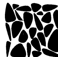
Figure 2. Schematic diagram showing interconnected pores (white space) in a rock. Black areas represent grains of minerals that make up the rock.
