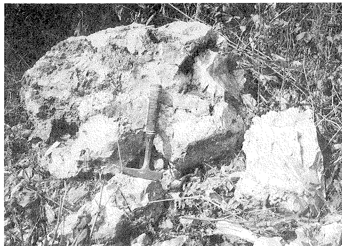
Figure 4. Honeycomb texture in residual chert boulder (visible at the left end of the rock). Such features contribute to the porosity of the chert. Geologic pick is ~1.1 ft long. (The location of the photograph is shown on Fig. 10.)
