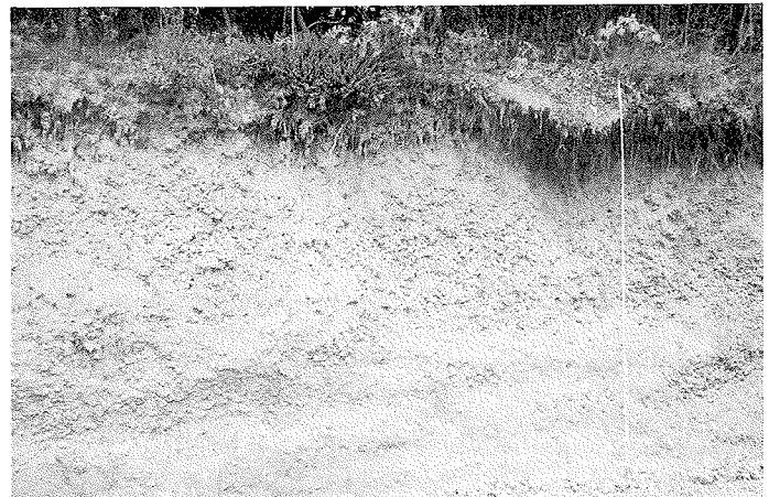
Figure 19. A 10-ft-thick horizon of moderate orange pink, silty clay and brecciated chert exposed in a road cut in a steep slope above the south fork of Clear Creek. The relationships of the materials in the exposure indicate that downslope creep is occurring. (The location of the photograph is shown on Fig. 10.)
