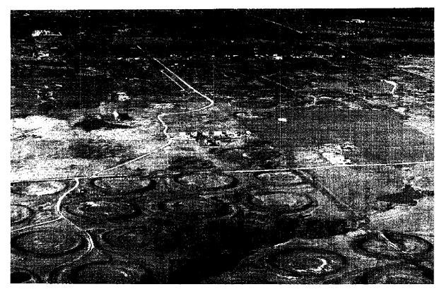
Figure 8. This February 1993 photograph (N<sup>1</sup>/<sub>2</sub> sec. 17 and S<sup>1</sup>/<sub>2</sub> sec. 8, T. 4 S., R. 3 W., looking northeast) shows an aerial view of an area that was formerly part of the Healdton oil field. Old sites of storage tanks, abandoned for more than 50 years, still show up prominently. Most tank sites are now used as pasture land, but some have been converted into stock or fishing ponds.
