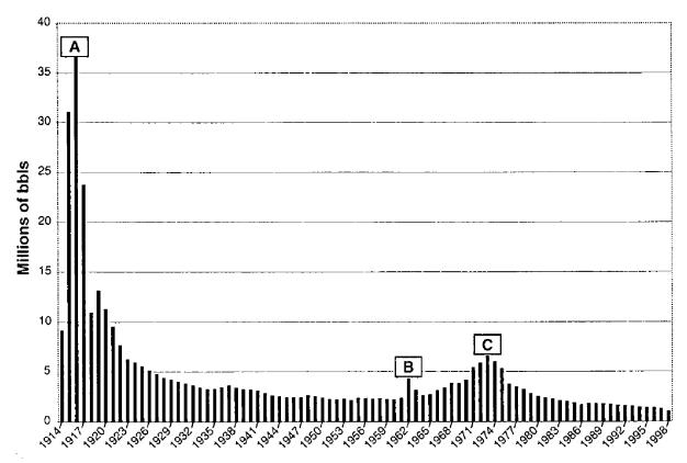
Figure 3. Annual oil production in the Healdton field, 1914–91: A—Maximum production in the boom period; B—Discovery of the Arbuckle Brown zone; C—Production peak that resulted from water flooding of the Healdton sand (Robinson, 1937; Petroleum Information Corporation, 1992).
