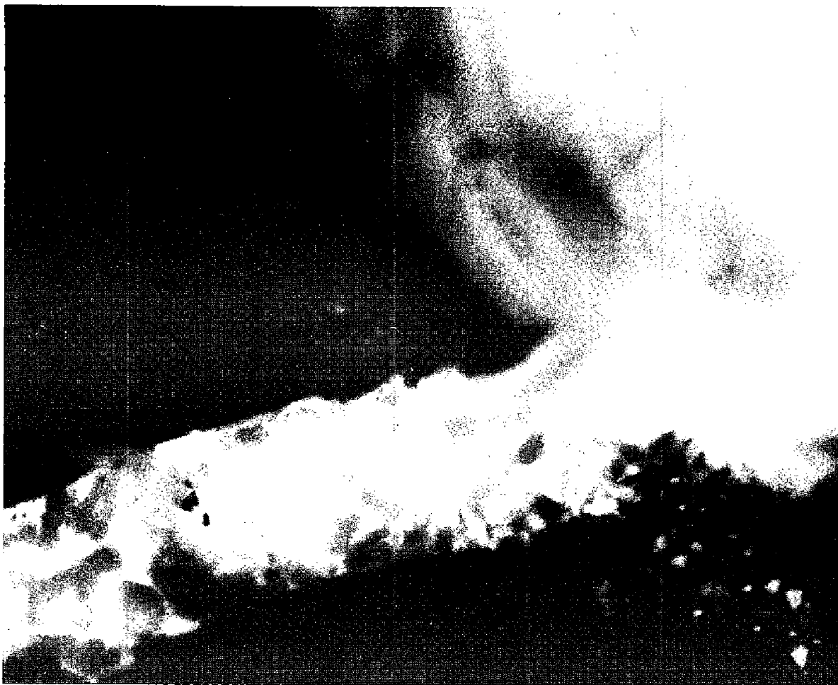
Figure 5. Photomicrograph showing flow and granular texture in secondary resinite (exsudatinite?) from the Mineral coal. Reflected light, blue-light irradiation, oil immersion, 500 ×, diameter of field 120 μm.
