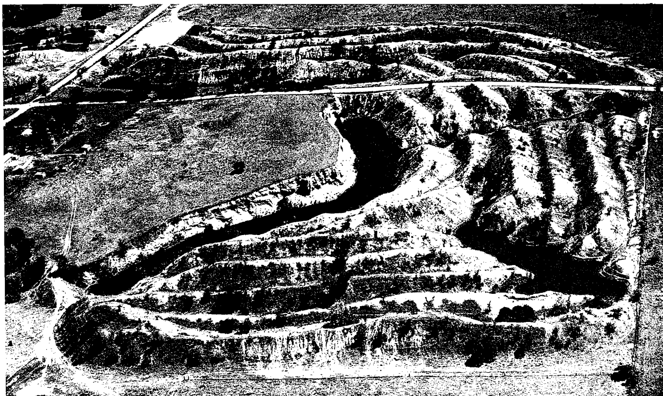
Figure 5. Aerial view of unreclaimed land mined for coal before passage of Oklahoma's reclamation acts. Vegetation is sparse, and water fills last cut (center) and part of abandoned haul road (lower right). Photograph taken in May 1971, looking south in sec. 21, T. 22 N., R. 16 E., Rogers County.
