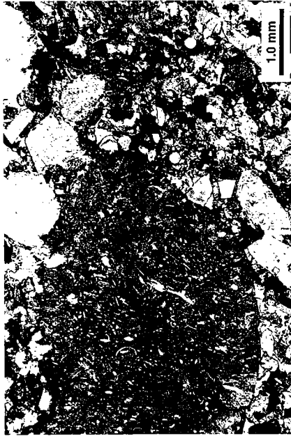
Figure 42. Photomicrograph of chert pebble where the grain matrix was selectively dissolved. Remaining light-colored material in grain is fossil debris. Exxon Sayre Ranch no. 1-35. Depth, 16,320 ft. Plane-polarized light.
