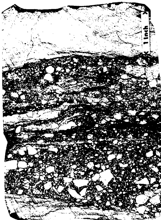
Figure 7. Cavern-fill parabreccia. Matrix-supported clasts of packstone and mudstone. Samson Wade core, depth 6,032 ft.
