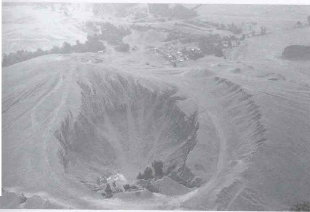
Figure 7. Aerial view of largest non-shaft collapse (2.60 acres), Blue Goose No. 1 Mine, 29N-23E-30(1511).
