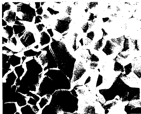
Figure 5. Scanning electron micrograph of whetstone novaculite showing sharp edges of quartz grains (SEM courtesy of W. D. Keller and George W. Viele, University of Missouri-Columbia).
