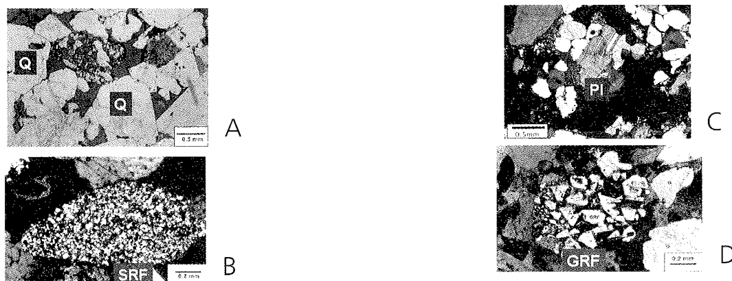
Figure 10. Detrital constituents in upper Morrow sandstones. (A) Quartz (Q) sand grains (plane-polarized light [ppl]). (B) Sedimentary-rock fragment (SRF) (cross-polarized light [cpl]). (C) Plagioclase (Pl) in fine- to medium-grained sandstone (cpl). (D) Granitic-rock fragment (GRF) (cpl).
