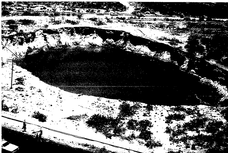
Figure 2. Aerial photograph of Wink Sink no. 1 on June 5, 1980 (photograph by R. W. Baumgardner, Jr.). Sinkhole reached 360 ft wide and 110 ft deep; depth to water surface is ~33 ft.
