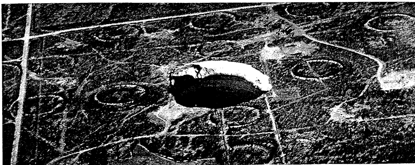
Figure 8. Aerial photograph of Wink Sink no. 2 in March 2003 (photograph by Jim Newman, Triple N Services, Midland, Texas). Sinkhole is ~780 ft by 610 ft. Viewed looking to the west, along the long axis of the sink (view shows 610-ft width). Each of the circular berms in the photo is ~300 ft in diameter.
