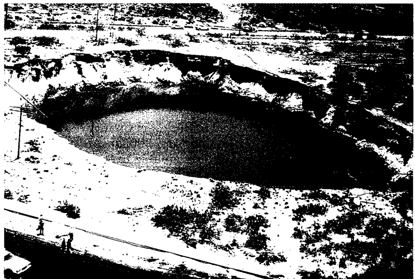
Figure 8. Aerial view of Wink Sink no. 1 in West Texas, shortly after its collapse in 1980 (photo courtesy of R. W. Baumgardner, Jr.). The sink, with a diameter of 110 m, formed at the site of an abandoned oil well.
