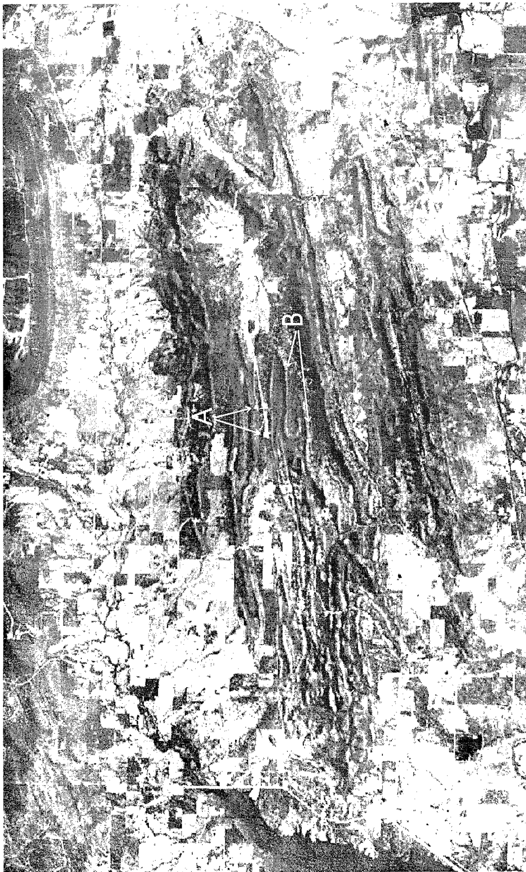
Figure 4. IRS LISS-3 satellite image, acquired March 22, 1997. The image shows the progress of GHK, Inc., at the time of image acquisition. Two well pads and the supply road can be seen clearly (A), and the image shows most of the folds in the Arkansas Novaculite south of the well pads (B). Image courtesy of Space Imaging, Norman Oklahoma.
