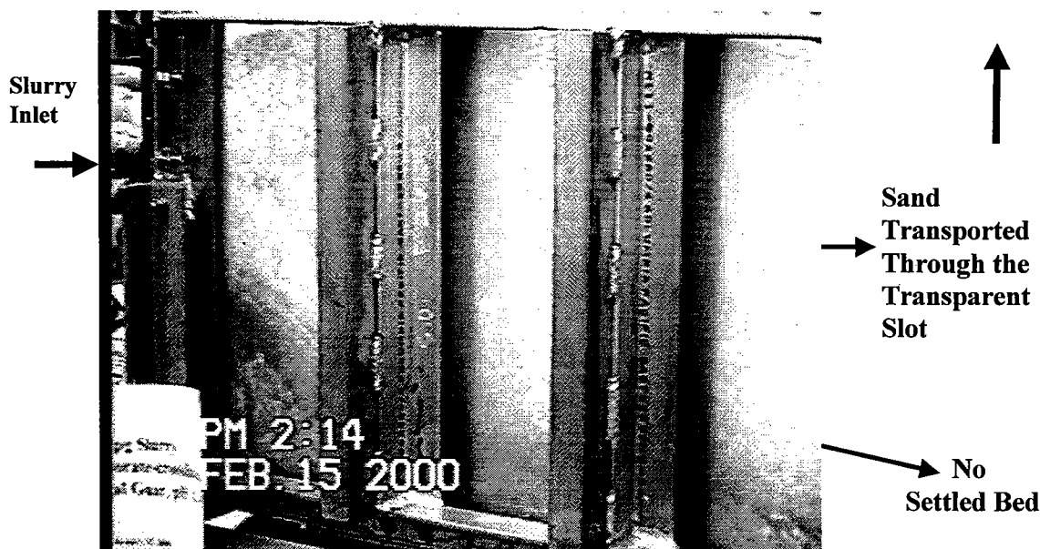
Figure 7. Proppant transport in transparent slot with 0.45-lb/Mgal borate-cross-linked guar gel.
