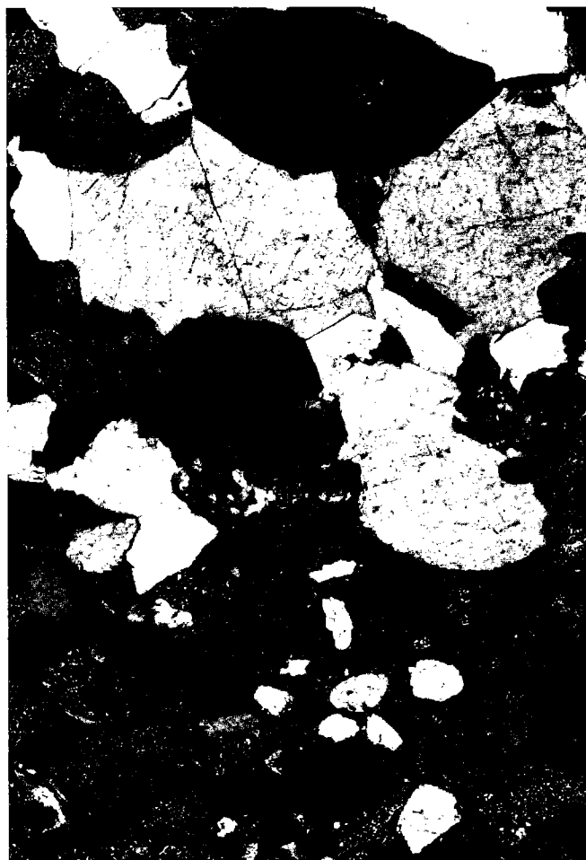
Figure 9. Photomicrograph (polarized light) showing the contact between an upper medium-grained gray-green sandstone with a substantial content of quartz grains and a lower fine-grained sandstone in which most of the grains are glauconite peloids. The upper sandstone was lithified by syntaxial quartz cement, whereas the lower sandstone was lithified dominantly by compaction. Field of view ~3 mm across.
