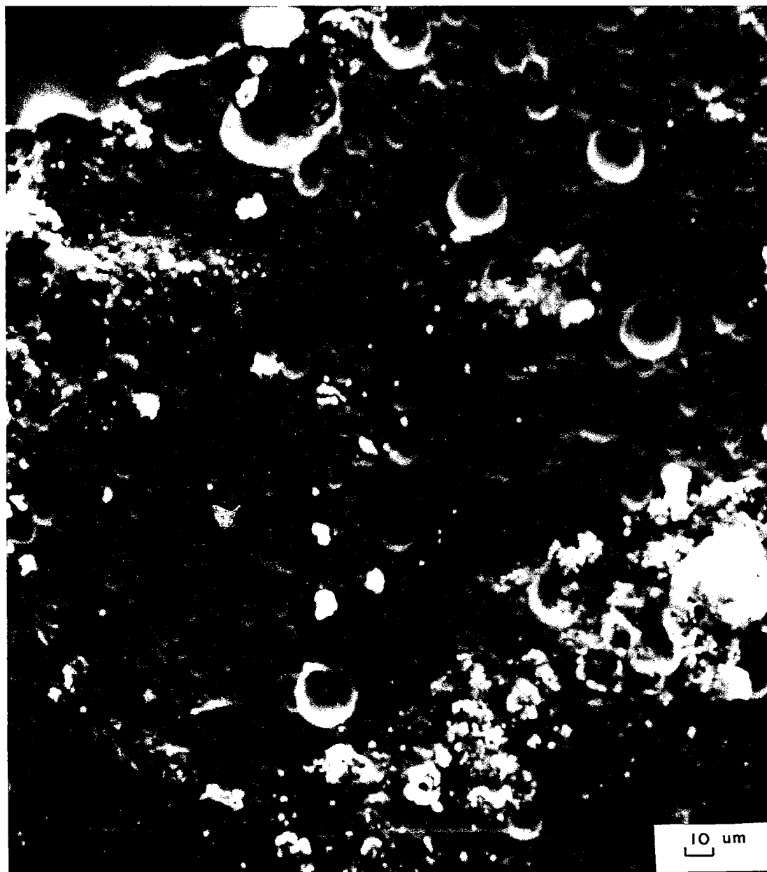
Figure 8. Scanning electron micrograph of surface of silica glass plate. All examples studied showed similar pockmarking by innumerable round depressions. (Micrograph by Bruce Cutler, SEM Laboratory, University of Kansas.)
