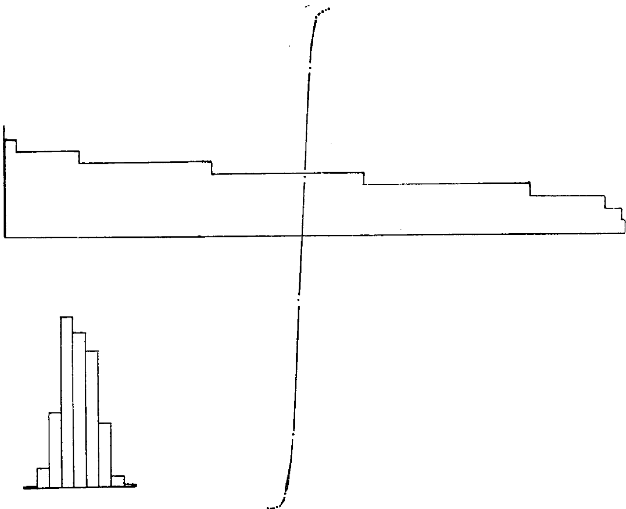
FIGURE 2. Histogram, cumulative percentage curve, and horizontal bar-graph showing the distribution of ground elevations in Seminole County. The data from which these figures were plotted are given on page 20. The horizontal bar-graph was constructed to show elevation along the vertical ordinate, and hence to represent graphically the actual average relief of the county.
