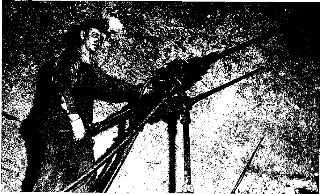
A. Drilling ore in the mine stope.
