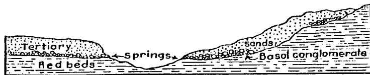
Figure 6. Ideal section of Tertiary springs—after Gould.
