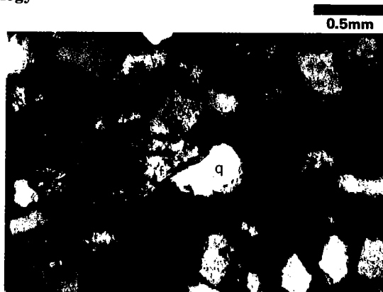
Figure 35. Photomicrograph of sandstone directly below Neva Limestone. The quartz-rich subarkose is primarily composed of subangular, well-sorted, fine-grained quartz (q) and feldspar (f). Crossed nicols.
