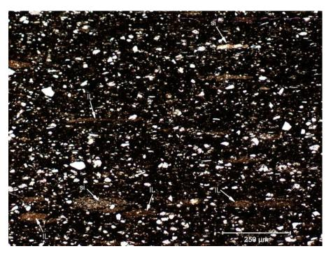
UW1 sample showing silicified Tasmanites; sample is 64% quartz and 21% clay. Silicic mudstone lithofacies.
